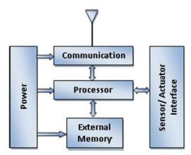
Fig (2): Architecture of WSN node
