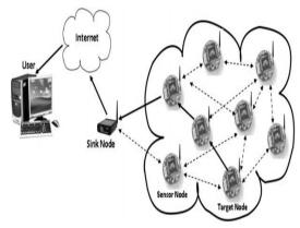
Fig(1): Wireless Sensor Network Architecture
